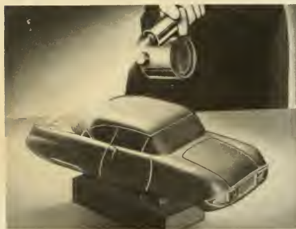
Use insect spray gun to lacquer model. Thin lacquer until it flows freely.
